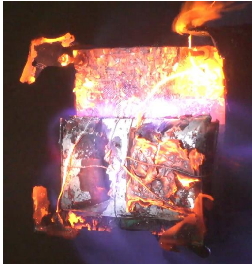
Figure 4: Removal of Aluminium from CubeSat Frame in Wind Tunnel Test
